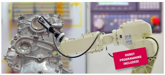
Static test systems with fixed cameras are usually inadequate for the quality monitoring of large, complex and varied assemblies. Modern image processing systems for test systems in modern production are increasingly used directly on the production line.
